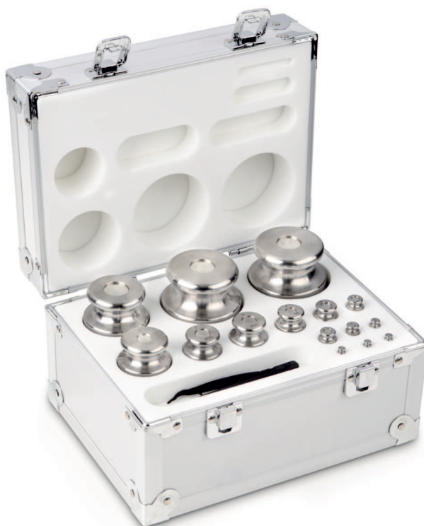
Weight set, F2, 1 g - 2 kg, Knob, stainless steel fine turned, in aluminium case
