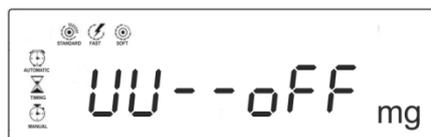
⇒ Choose the data transmission type, pressing **ENTER**, switch it on/off using the navigation buttons **↓** **↑**.
