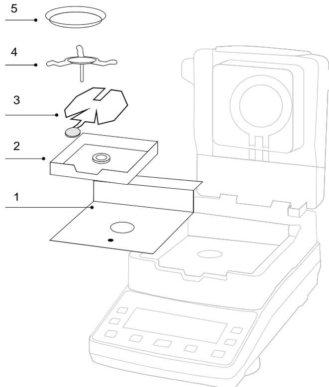
1. Put heat shield into the sample chamber.
