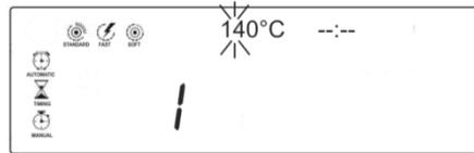
⇒ Use the arrow keys   to enter the desired test temperature. For the first or the first two digits select a value and confirm by .
