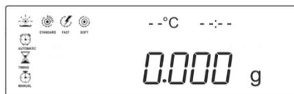
To **switch off** press the ON/OFF button, the display disappears.
