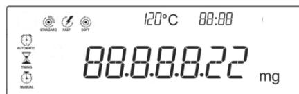
„8.2X“ will be displayed. If not, separate device from power supply and restart step two.
