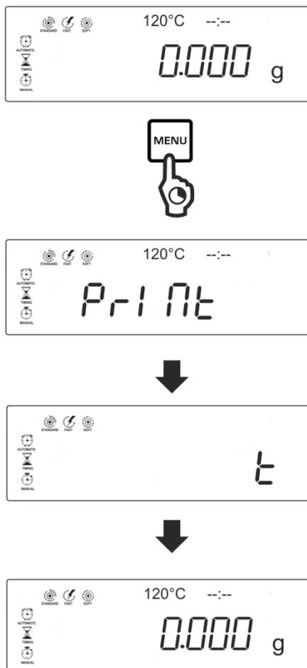
This is the starting/finishing time of continuous data transmission when the measurement is started/completed.
