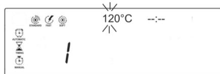
⇒ Using arrow keys   select the desired value for the last digit.
