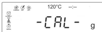
⇒ Wait until the weighed value for the required adjustment weight appears flashing.
