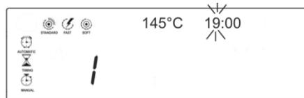
⇒ Using arrow keys  , select the desired value for the next digit and confirm by , the next digit is flashing. Repeat this procedure for all digits.
