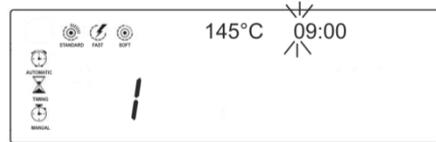
⇒ Using arrow keys  , select the desired value for the first digit and confirm by , the next digit is flashing.
