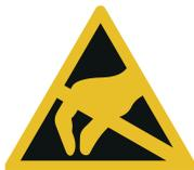
Electrostatically endangered structural components
