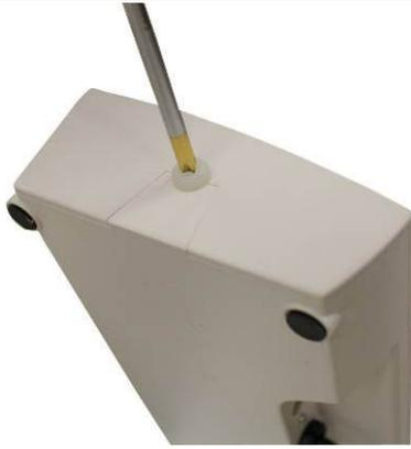
Take a screw driver and remove the plastic covers from both sides of the display unit.
