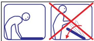
When installing or transporting balances with large and heavy platforms (weighing plate folded upwards), ensure that the balance does not fall over or gets damaged.
