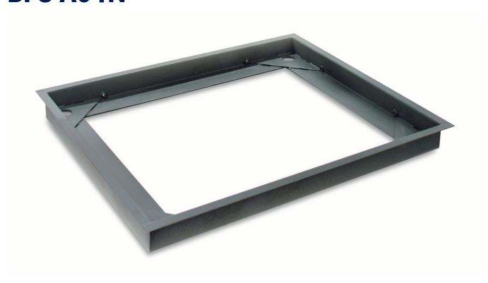
Stable pit frame for weighing bridge installation, allowing for easy access, W×D×H 1335x1585x80 mm, for models with weighing plate size B 1500×1250×80 mm, must be ordered at purchase
