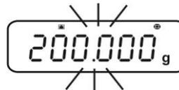
If the value shall be changed, press **MENU**, the active digit flashes. Carry out the desired setting using navigation buttons
