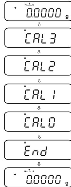
⇒ After successful adjustment the balance automatically returns to weighing mode.
