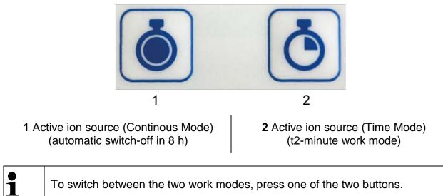
To switch between the two work modes, press one of the two buttons.
