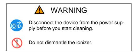
Do not use any aggressive cleaning agents (solvents etc.) for cleaning. Use solely a cloth with a mild soapy water. The liquid must not penetrate inside the device, use a soft cloth to wipe the device dry after cleaning.
