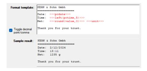
Functions are used to round the weighing value and remove the digits part of the PC time.
