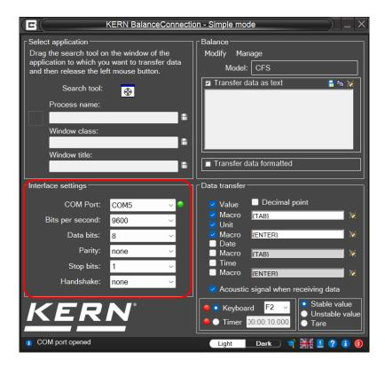
The balance must be connected to the PC via a serial cable. Prior to transferring data, you must ensure that the same interface parameters are set on the balance and the PC. Select this program item for this purpose.
