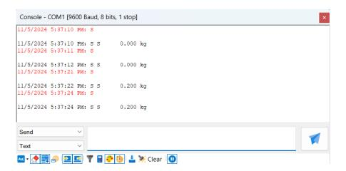
The terminal displays the data received from the connected device and the data transmitted to the device by the software as raw data. In the toolbar you can choose between a variety of display options.
