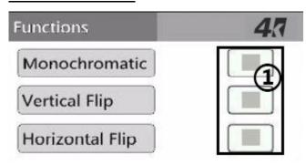
① Switching the grey scale, vertical flip and horizontal flip functions on/off
