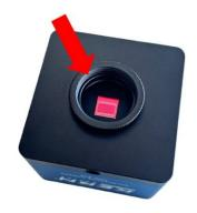
There is a standardised C-mount thread under the cover. This is used for mounting on a C-mount adapter.
