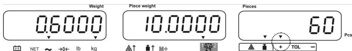
The information if the goods to be weighed are within the tolerance limits, can additionally be given by an acoustic signal (menu item „BEEP“, see chap. 13.2)
