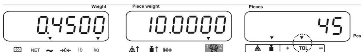
Display of tolerance mark ▼, if weighing goods above the specified tolerance:
