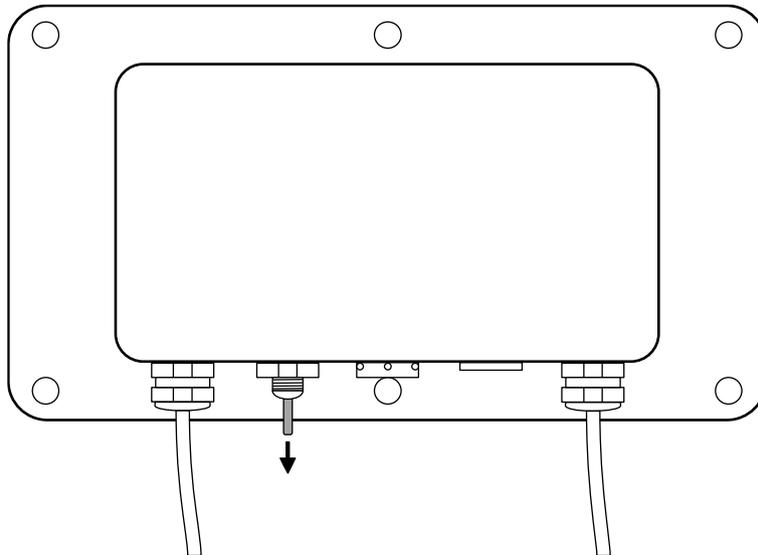
8. Use the cable cores to guide the interface cable through the sealing cap.
