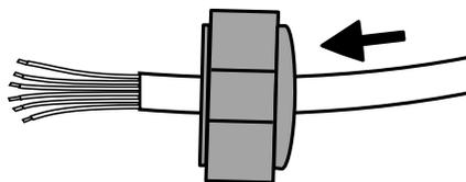
9. Use the cable cores to lead the interface cable through the cable gland from the outside so that the cable cores are inside the enclosure.
