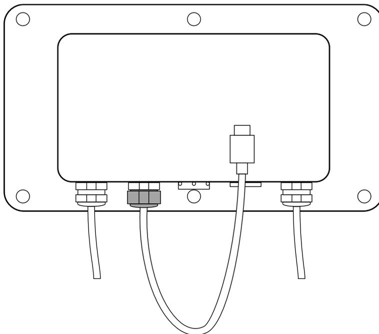
12. The interface cable must be passed through the module's cable tie.
