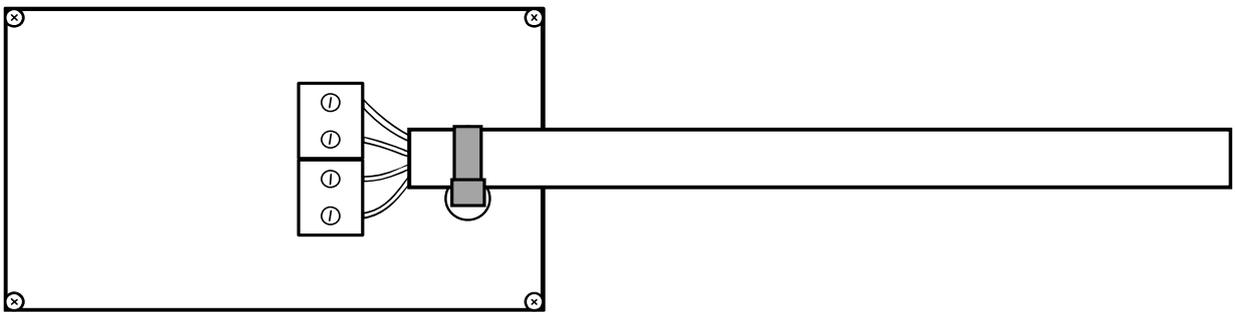
**16.** Place the ferrite core around the cable and close it.
