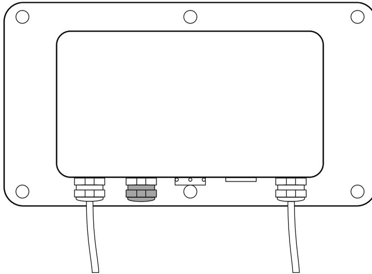
7. Remove the sealing pin of the cable gland.
