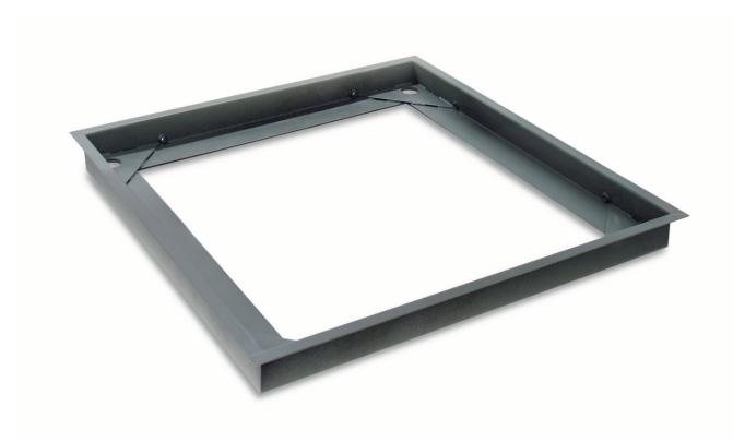
Stable pit frame for weighing bridge installation, allowing for easy access, W×D 1090x1090x86 mm, for models with weighing plate size 1000×1000×80 mm, must be ordered at purchase
