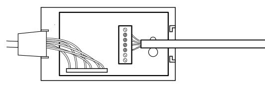
6. Insert the lower part of the cable gland into the guide of the module enclosure and place the cable into the cable gland.
