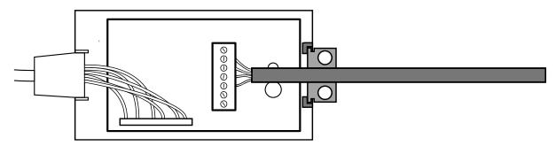
7. The upper half of the cable gland is screwed onto the lower half.
