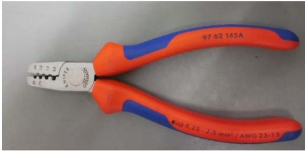
Use the smallest possible wire-end ferrules and use a wire end ferrule crimper to press them onto the cable (See illustrations)
