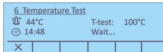
5. After 15 minutes the test is finished, an acoustic signal sounds. Compare the test temperature with the displayed temperature of the DLB-A01N. If the two values do not match, we recommend a temperature adjustment, see chap. 2.2
