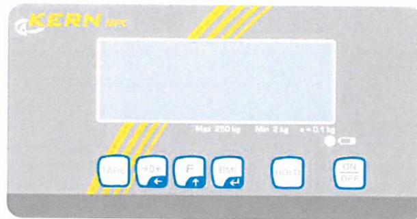
**Figure 4** Front layout of indicator on MPC
