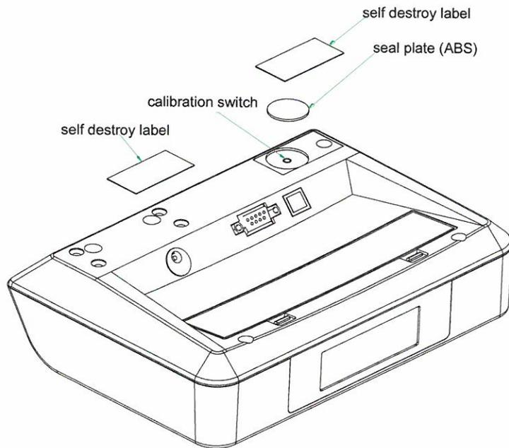
**Figure 13** Sealing of indicator for model MPE.
