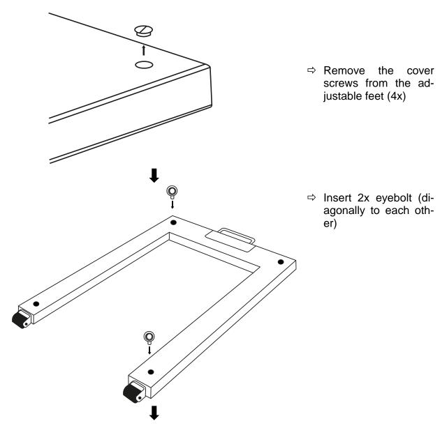
⇒ Have the weighing platform lifted by qualified personnel using a lifting aid (crane or similar)
