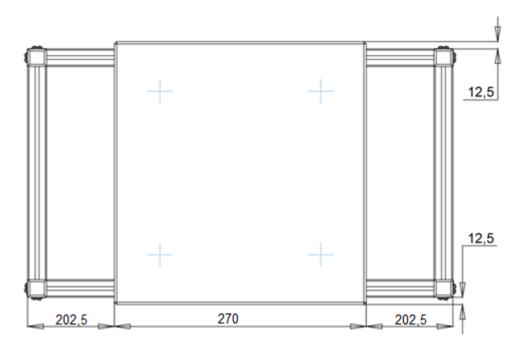
7. Place the granite block on top and centre it as precisely as possible.
